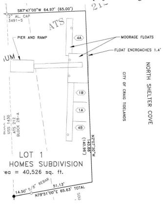
5'x38' finger. The proposed project appears to align the floating main dock parallel to the existing upland and the fingers on both sections perpendicular to the upland to accommodate head in moorage for vessels.
