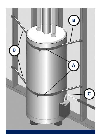
Wrap a 1½" wide, 16-gauge-thick metal strap (A) around the top of the water heater and bolt the ends together. Do the same about 1/3 of the way up the side of the water heater. Take four lengths of EMT electrical conduit, each no longer than 30". Flatten the ends. Bolt one end to the metal strap (B). Screw the other end to a 2" by 4" stud in the wall using a 5/16" by 3" lag screw. Be sure a flexible pipe (C) is used to connect the gas supply to the heater.
