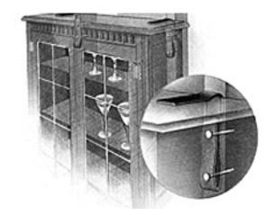
Bookcases and shelving should be anchored with brackets or flexible fasteners to an adjacent stud wall, or concrete or masonry wall. Any connections to stud walls must engage the structural studs.
